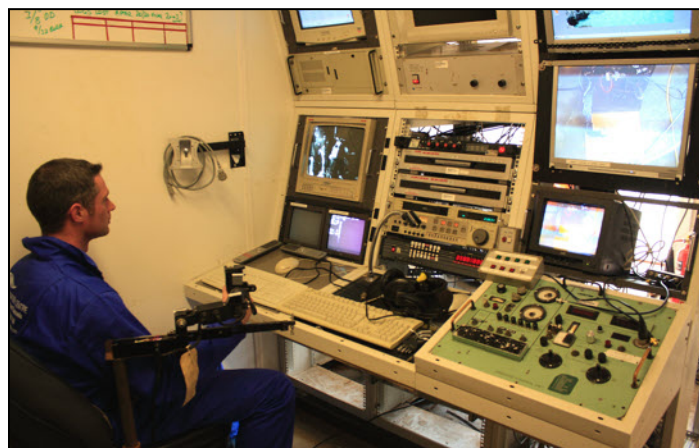
The Centre's ROV course includes training on a 7-function master/slave manipulator arm
