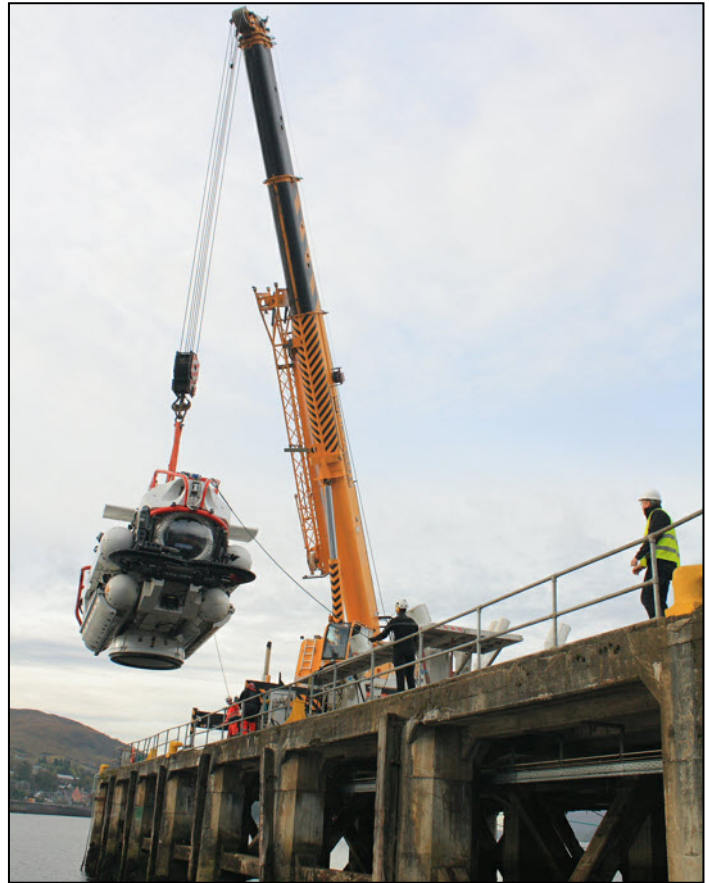
The NSRS being lowered into Loch Linnhe from the Centre's pier
