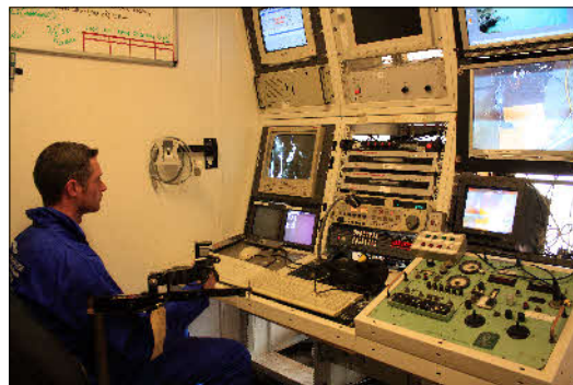
Middle: Operating the Perry Slingsby TA009 manipulator from the control cabin
